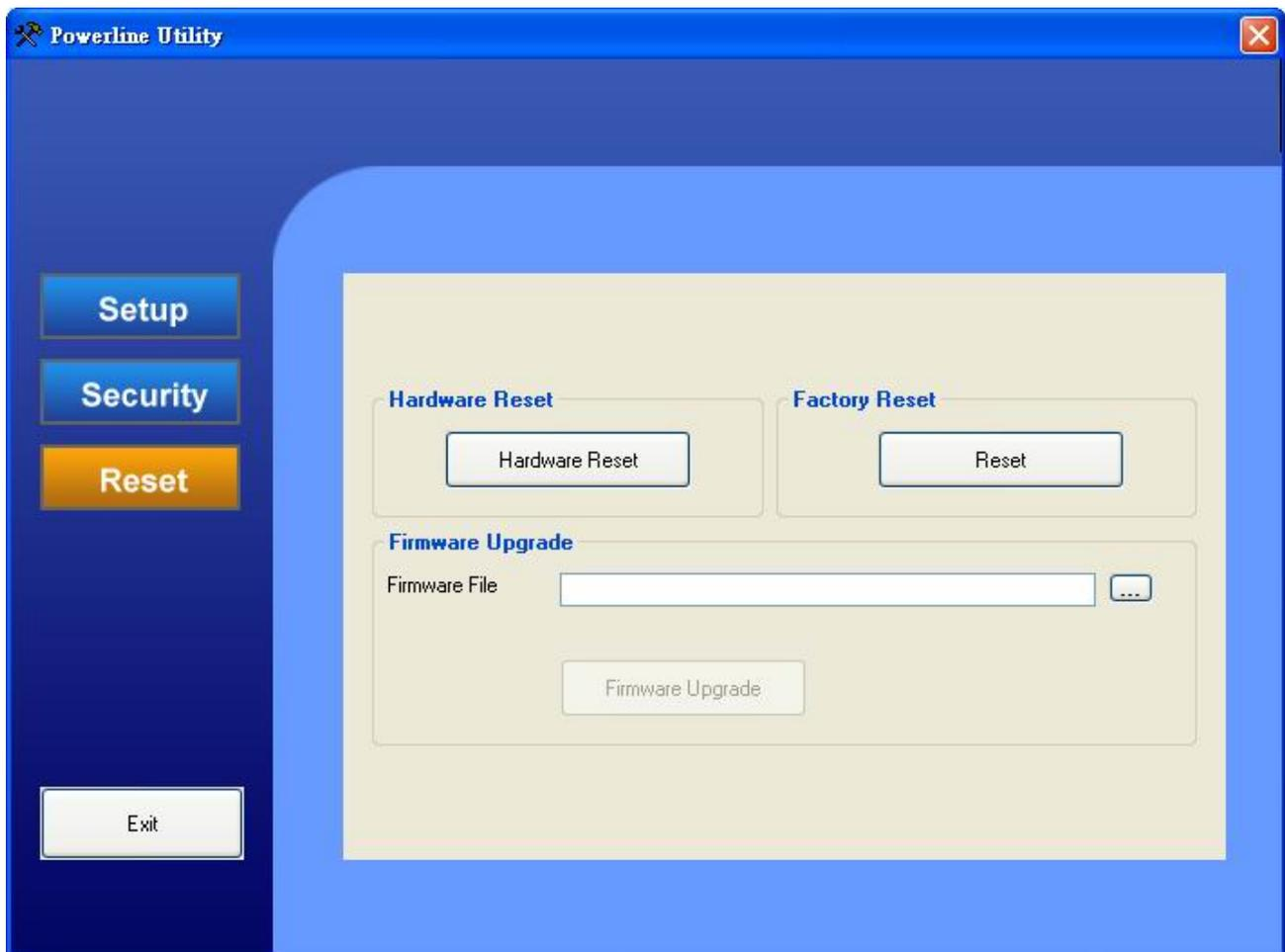
4. Select the “**ETH Connected Node**” and click the “**Factory Reset**” button.
