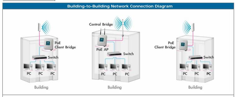
The UOW2000-AP67 operates in AP mode or remote Bridge mode, and connect to UOW2000-AP/CB to construct point-to-point as well as point-to-multipoint topologies, for maximum flexibility in configuring building-to-building networks and WISP functions
