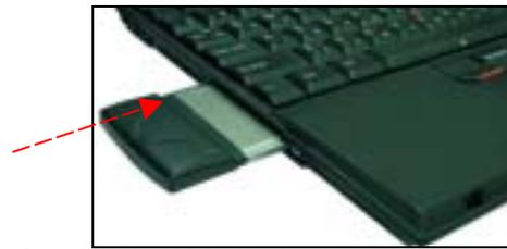
When The **Super G Wireless PC-Card** has been inserted into a 32-bit Card bus slot, the **Found New Hardware** screen appears. Continue with the installation and the screen below should appear. Click on **Yes** to proceed with the installation
