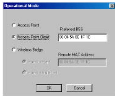
**Access Point Client:** In this option, the Access Point can be a base station in a WLAN system, but also as a client station to communicate with other stations in the WLAN system. In this option please type in the “Preferred BSS” for the WLAN network system which it wants to join in.
