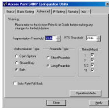
**Fragmentation Threshold:** The value indicates how much of the network resources devoted to recovering packet errors. The value should remain at its default setting of 2432 bytes. If you have decreased this value and experience high packet error rates, you can increase it again, but will likely decrease overall network performance.
