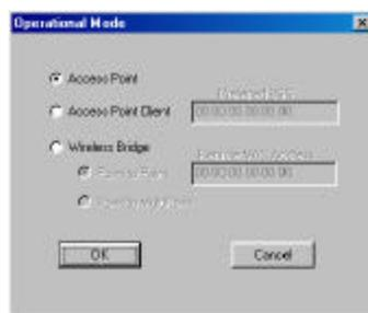
**Access Point:** This mode provides access for wireless stations to wired LANs and from wired LANs
