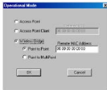
**Wireless Bridge:** This mode allows the connection of one or more remote LANs with a central LAN, creating thus an extended single virtual LAN. In this way, any station of the Remote LAN can successfully communicate with any station of the central LAN, as if all of them belonged to the same physical LAN. Wireless station can't associate with wireless bridges. The Access Point conducts the designated traffic to the appropriate wired or wireless station.
