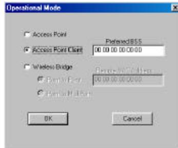
**Access Point Client:** In this option, the Access Point can be a base station in a WLAN system, but also as a client station to communicate with other stations in the WLAN system.
