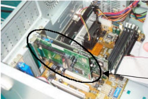
Plugging the PCI-to-PCMCIA adapter to your computer's PCI slot.
