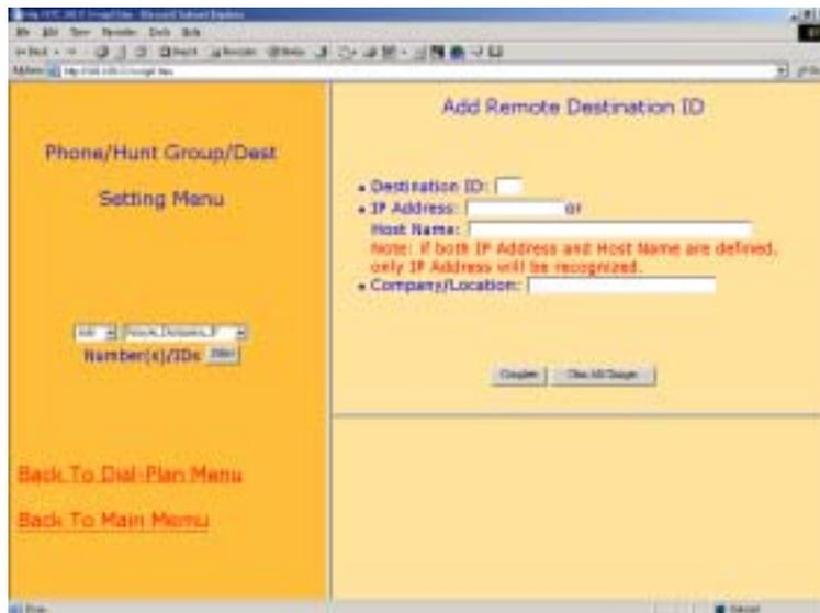
The information associated with “Destination ID” and “IP Address” of the remote Gateway should be filled in. Click “Complete”. The newly added remote IP address will be displayed for confirmation as follows:
