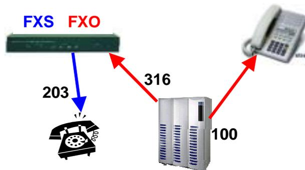
Pick up your extension handset, for example, 100 and dial '316'. After two rings, you should hear a dial tone. Now dial '203' the telephone connected to the ITG FXS port should ring.
