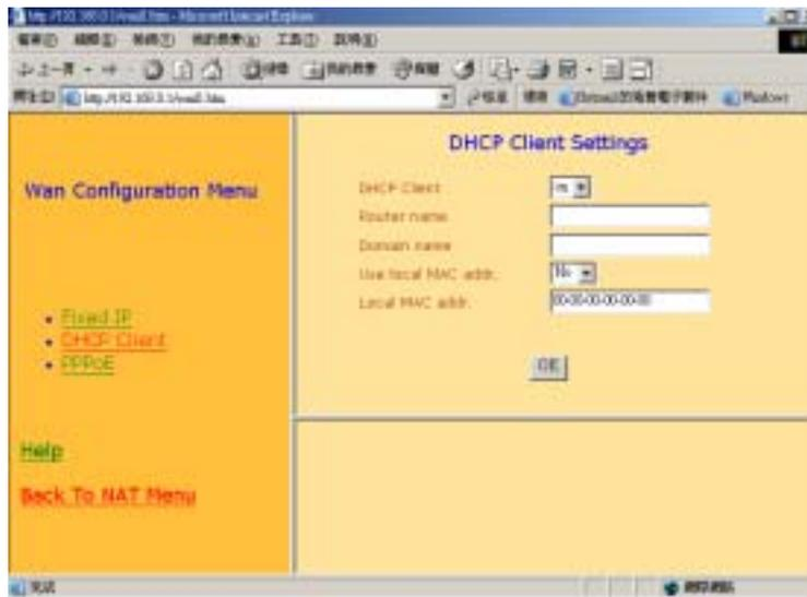
At “DHCP Client” field, select “on” for enable DHCP client.
