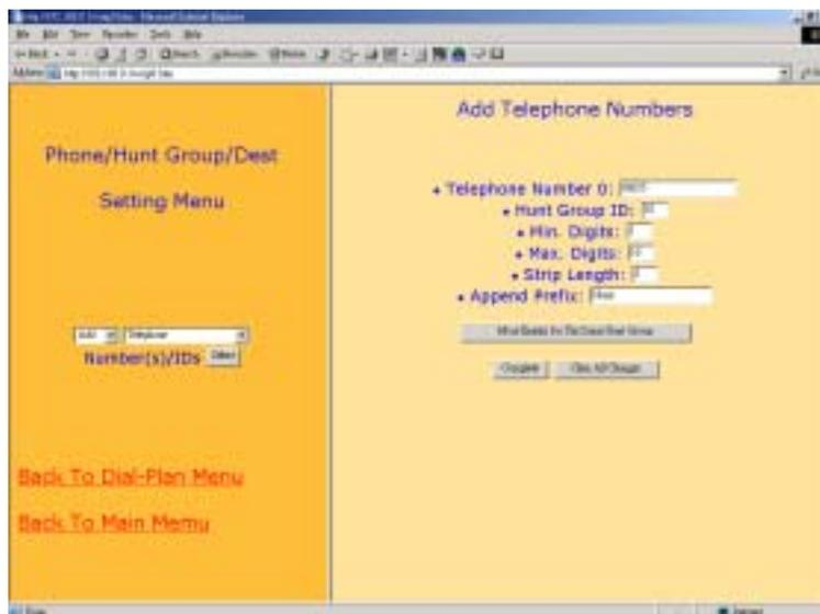
Fill in the information associated with "Telephone Number", "Hunt Group ID", "Min. Digits", "Max Digits", and "Strip Length". Make sure the above data is correct then click "Complete".
