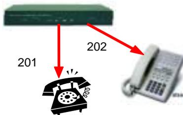
Suppose two telephones are connected to two of your ITG FXS ports, say port 1 and port 2 respectively, you just pick up phone 1 and dial '202' directly, phone 2 should ring.
