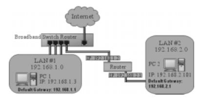
In the above diagram, PC2 in LAN#2 is connected to the Broadband Switch Router via another router while PC1 in LAN#1 is connected to the Broadband Switch Router directly. Without configuring the Static Routing function, the two PCs would not be able to communicate with each other.
