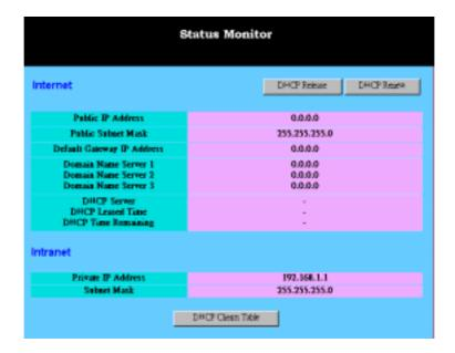
Internet This section shows the IP settings status of the router as seen by external users of the Internet. If you selected "Get IP Address Automatically", "PPPoE", or "PPTP" in the OnePage Setup, the "IP Address", "Subnet Mask", "Default Gateway", and "Domain Name Server" (DNS) will show the information retrieved from the DHCP server or ISP which is currently being used. If you selected "Static IP" in "One Page Setup: Public IP Address", the information will be the same as your input.
