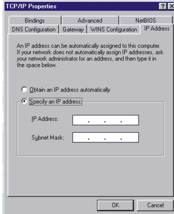
4. Fill in the IP address. State the subnet mask to be 255.255.255.0.
