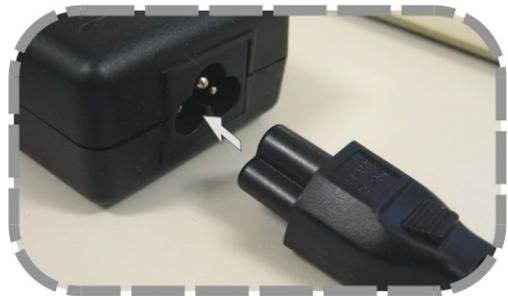
2. Connect the connector end to the device and the plug to an outlet.
