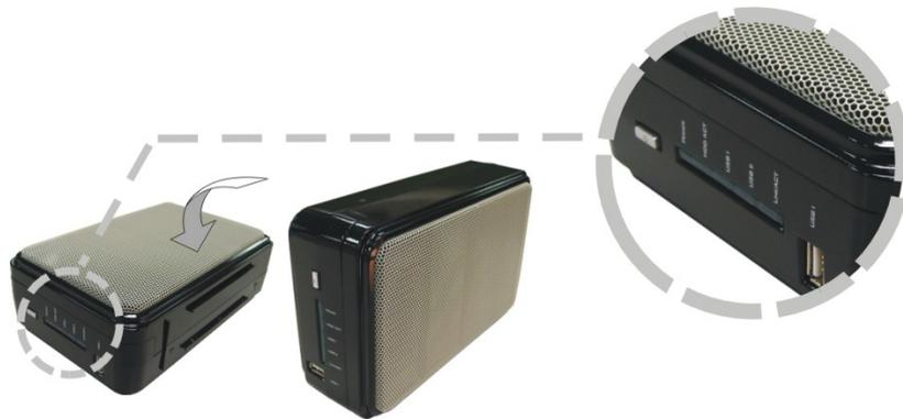
2. Unscrew the screws on both the top and bottom side of the device.
