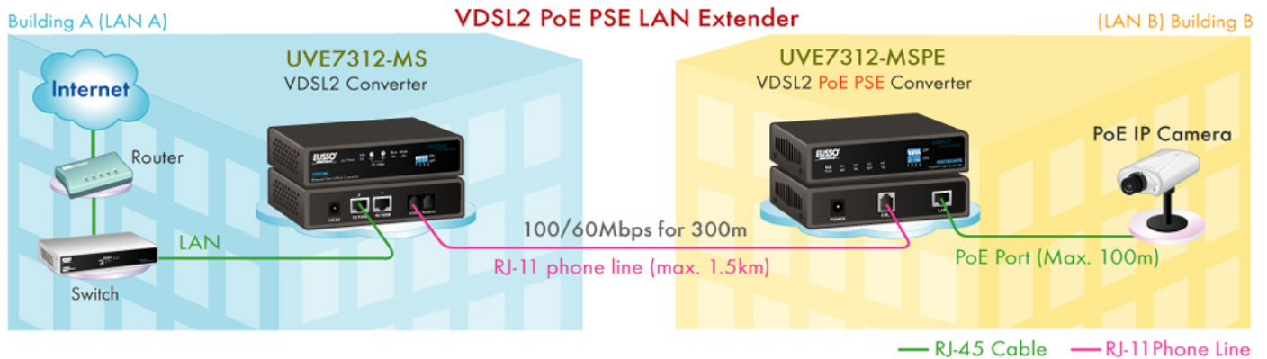
Ethernet over VDSL2 PoE (PSE) Converter Application Diagram
